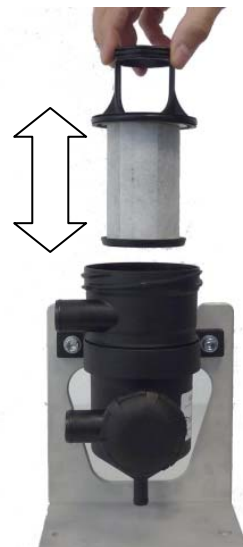
Fig. 15 Changing oil separator of ProVent 200
