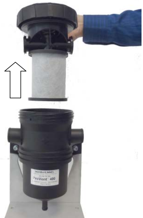
Fig. 18 Removing oil separator of ProVent 400
