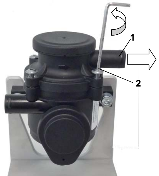
Fig. 10 Detaching lid of ProVent 100
