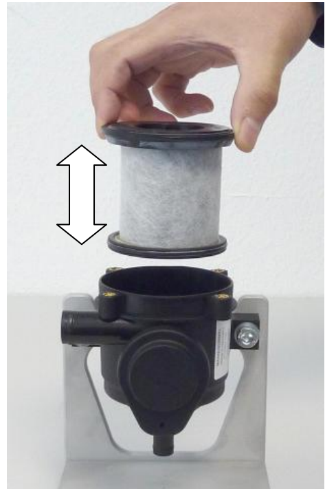
Fig. 11 Changing oil separator of ProVent 100
